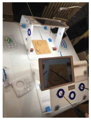
Figure 1. Structure of the laparoscopy simulator
